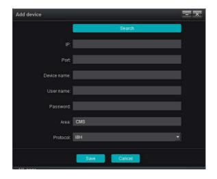
Select the protocol, which register protocol is for the active registration agreement, this protocol is develop by our RD team and it need the support of the front-end device. I8H protocol also is develop by our RD team, currently all our front-end device support this protocol .I8 protocol also is develop by our RD team. For the old version which not support I8H, Can connect through I8 protocol.
