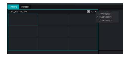
The decoding mode represents the decoder's current decoding capability, the decoder shown in the picture supports three decoding modes, 16ch 720x576, 9ch 1280x960, 4ch 2048x1536 (Notice: number means the highest decode resolution, for example under 9ch mode, highest decode resolution is 1280x960, different model decoder will have different decode capability). Front-end IPC resolution not higher than current decoding mode's solution limitation, the display can be decoded normally.
