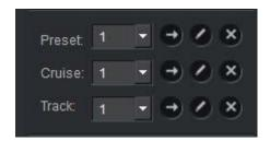
Preset point: the PTZ machine rotates to the point where preset points need to be set. Click on the PTZ you can set preset
